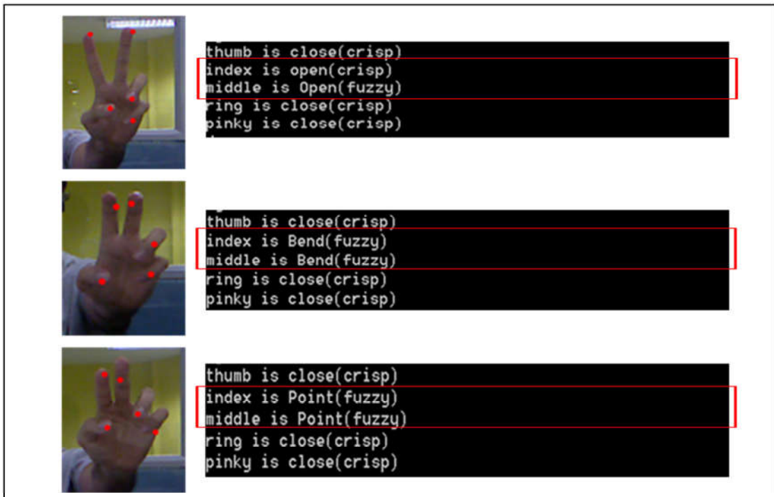
Figure 3.20 Finger shape feature classification using fuzzy logic.
