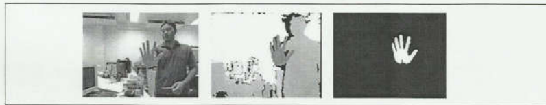
Fig.2. RGB-D Information: (a) colour image (b) depth image (c) hand segmented
