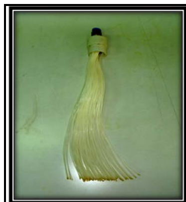
Figure 4.2 The hollow fibre membrane module (PVDF membrane).
