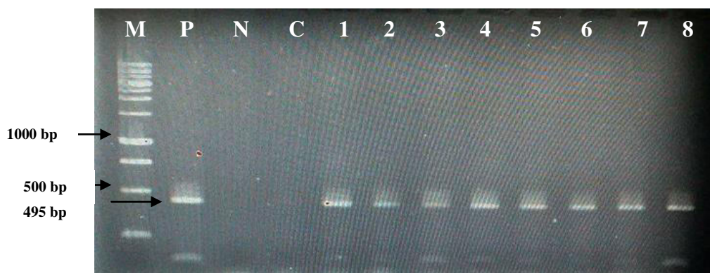
Figure 19 PCR analysis of genomic DNA of the putative transgenic callus to detect the presence of the GUS gene. The red arrow indicates the expected PCR product of the GUS gene. Lane M: marker 1kb size, P: positive control, N: negative control, 1-8: lines of transformed callus
