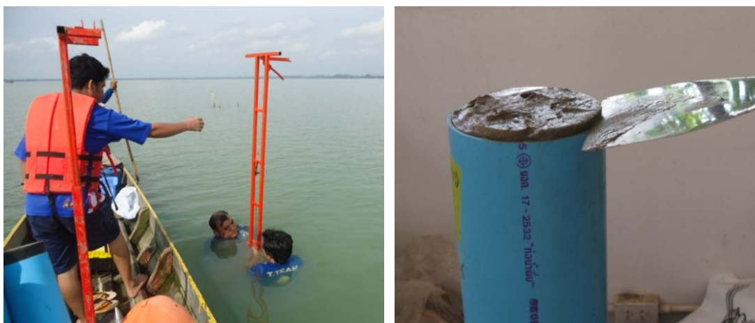
Fig. 2 Photographs showing (a) scenery of the study lagoon during sediment core sampling, and (b) slicing of an 0.5 cm thick layer from extruded sediment core, using a metal blade in the laboratory.
