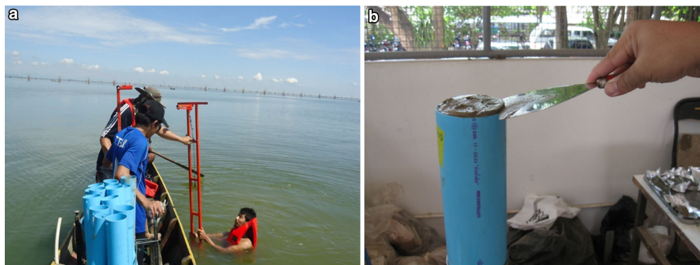
Fig. 3 Photographs showing a panoramic scenery of the study lake during sediment core sampling and b slicing the extruded piece of sediment core 0.5 cm thick using a metal blade in the laboratory
