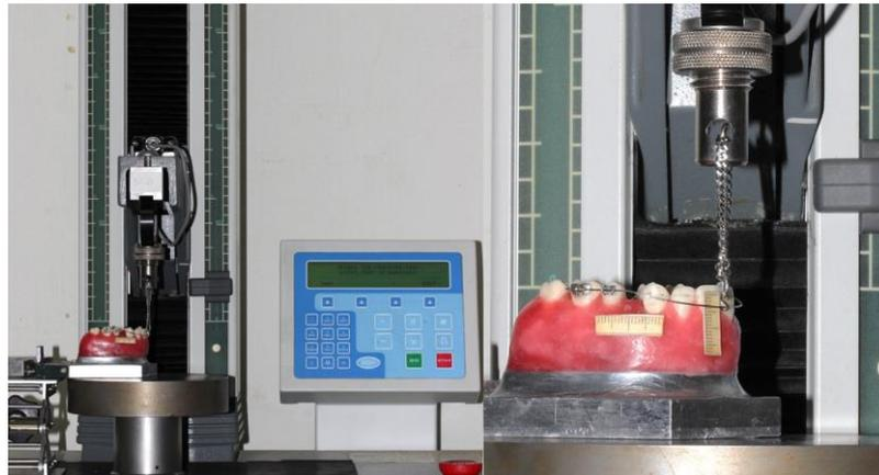
**Fig. 14** Universal testing machine and testing method
