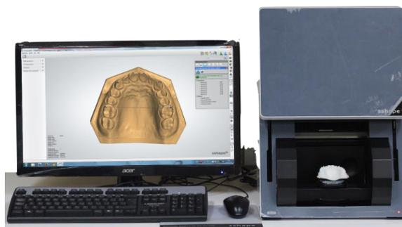
**Fig. 20** Generating the 3D digital model with a specific 3D scanner (3Shape R700<sup>TM</sup>)
