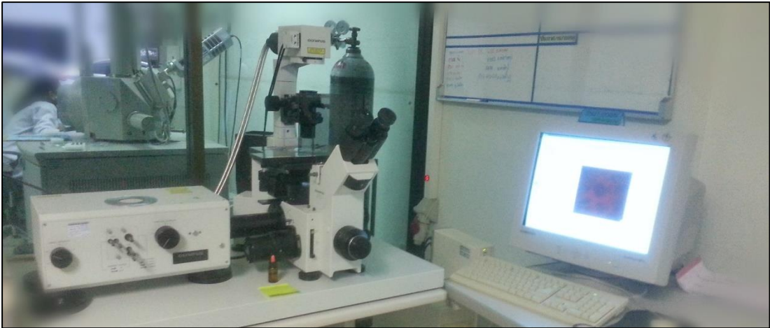
Figure 12. Confocal Laser Scanning Microscope (Model FV300 equipped with IX-70 Microscope, Olympus, Tokyo, Japan).
