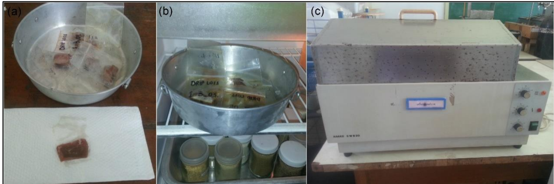
Appendices 1. 3. 1. Drip loss and cooking loss determination procedure. (a) cut muscle sample was blotted with towel paper and put in sealed plastic bag, (b) drip loss samples were stored in 4°C and (c) water bath that was used for cooking loss determination.
