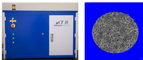
Fig. 6 Micro-CT35 scanner and 3D- reconstruction of the half of calvarial specimen.
