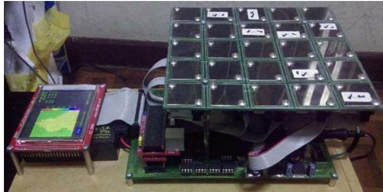
Figure 17. The laboratory prototype multi-plate ion balance analyzer.
