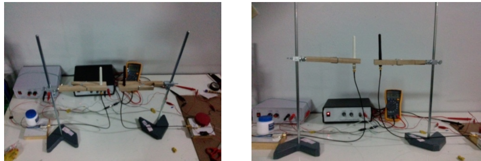
Fig. 3.2 The receiving and transmitting system using dipole antennae
