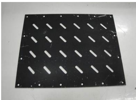
(ช) AR=4 , \theta = 45^\circ , Inline arrangement
