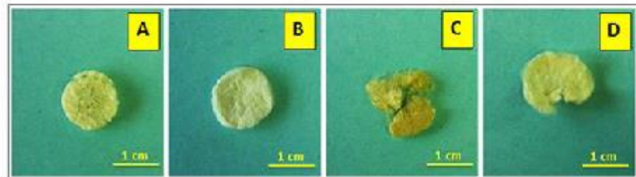
Fig. 5. Scaffolds after degradation with lysozyme at 4 weeks: A) silk fibroin scaffold, B) collagen coated silk fibroin scaffold, C) chitosan scaffold, D) collagen coated chitosan.
