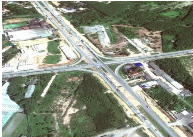
Figure 2.3 At-grade intersection type (example)
