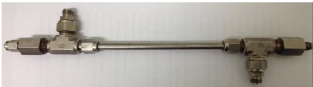
Figure 1 Lab-scale hollow fiber membrane module
