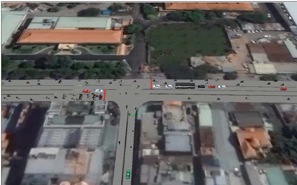
Figure 5.24 Simulation process of current traffic situation at black spot
