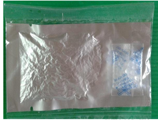
Figure 22 A. aceti TISTR 102 starter powder in vacuum aluminum-sealed pouch and packed with silica gel
