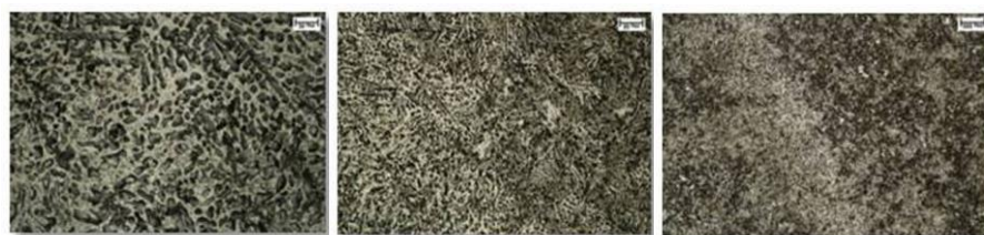
Fig.5 The microstructure of CLC Sn-50%Zn alloys at 50°C (a) 5x, (b) 20x and (c) 50x
