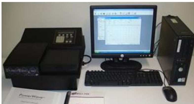
**Figure 3.10:** Microplate reader (Bio-Tec instruments, Inc., U.S.A) using absorbance value at 515 nm
