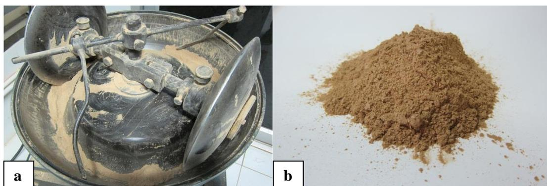
**Figure 3.3:** The grinder machine (a) and *E. elatior* rhizome in powder form (b)
