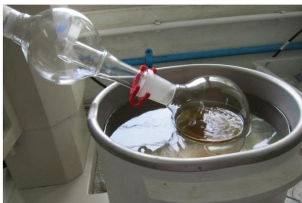
**Figure 3.6:** EtOH was removed from the EtOH extract using rotary evaporator at 45°C under vacuum
