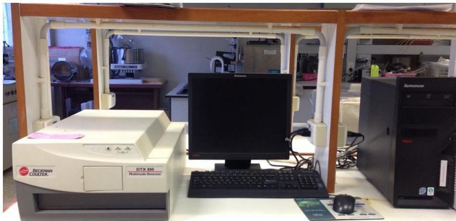
**Figure 4.5:** Microplate reader (Beckman Coulter, DTX 800, Austria) used for measuring the absorbance of enzyme activity testing
