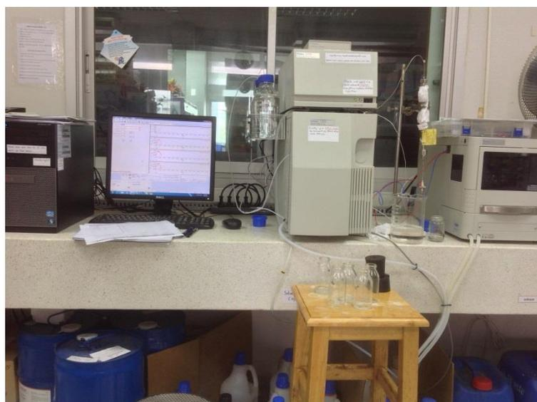
**Figure 4.14:** Reversed phase HPLC column chromatography used in purification processes
