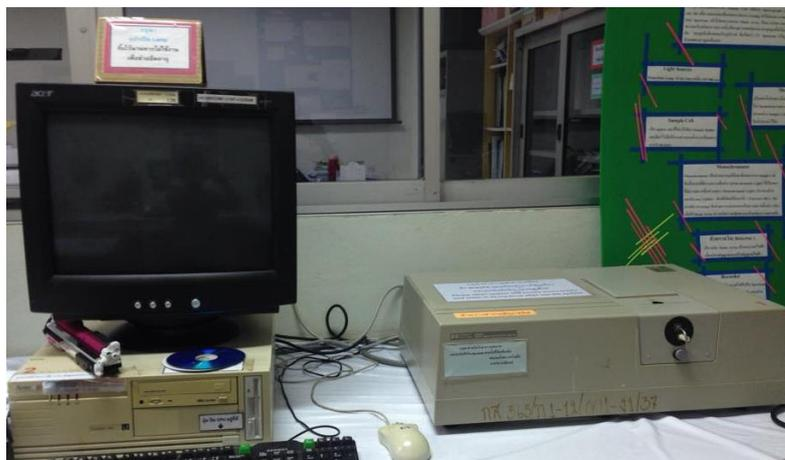
**Figure 3.9:** UV-visible spectrophotometer (Hewlett Packard 8452A, Diode Array Spectrophotometer, U.S.A) used for measure the absorbance at 515 nm for preparing the DPPH solution in a range of  $1.1 \pm 0.02$
