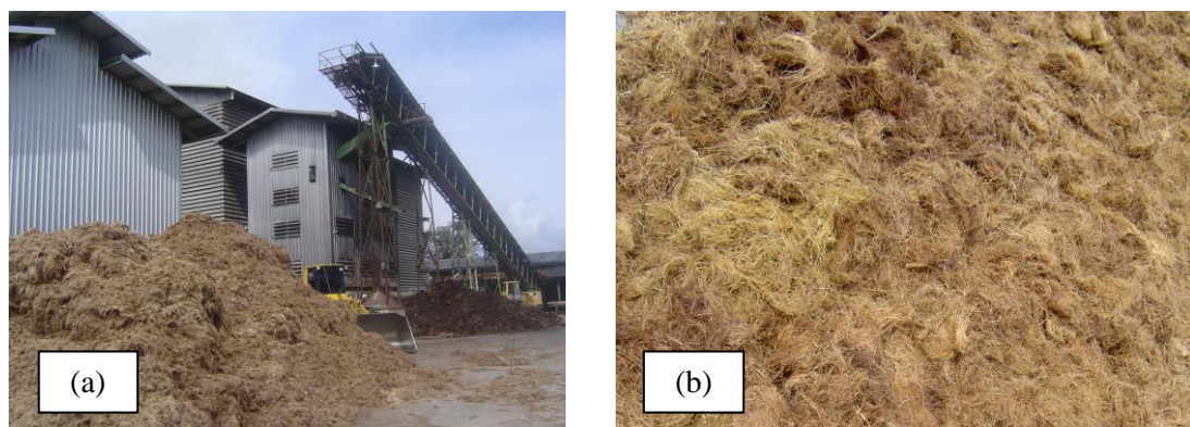
Figure 2-4 EFB biomass from oil palm mill industry (a), and lignocellulosic fibre of EFB (b)
