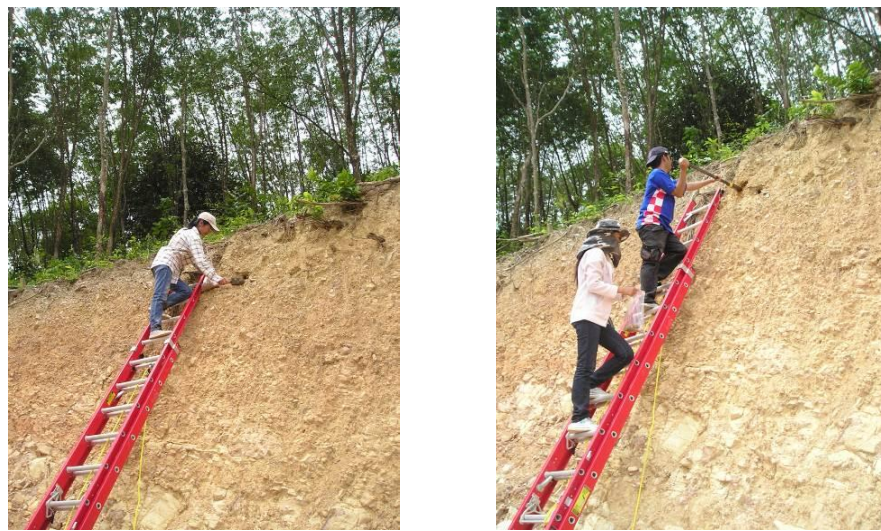
Figure 2.3 Samples of unconsolidated sediments collected by tool in-situ and samples were put in a plastic bag.
