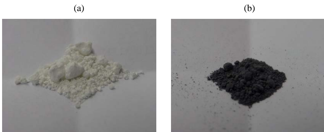
Figure 20 The images of two kinds of the powder (a) the commercial AgCl powder and (b) the flower-like Ag/AgCl powder.
