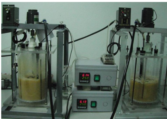
Figure 26. The set apparatus for T. spathulata JU4-57 in a stirred tank bioreactor under batch and fed-batch fermentation.
