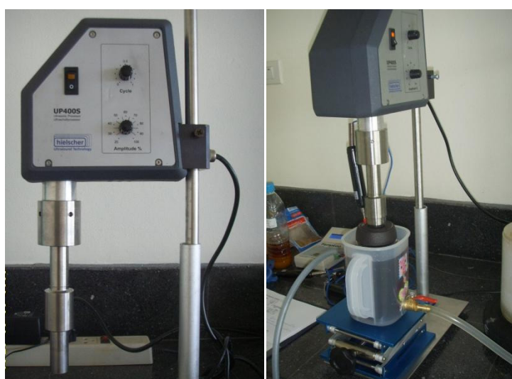
Figure 2.2 Equipment setup of the batch esterification
