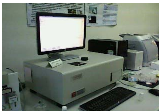
Figure 3.6 Zeta potential analyzer (Model Zeta PALS, Brookhaven Instrument, USA) used size stability determination of liposome during storage.
