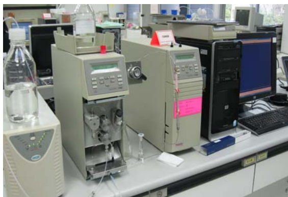
Figure 3.5 High performance liquid chromatography (HPLC) systems used for determination of rhinacanthin-C stability in liposome (Thermo-isoretic pump, USA).
