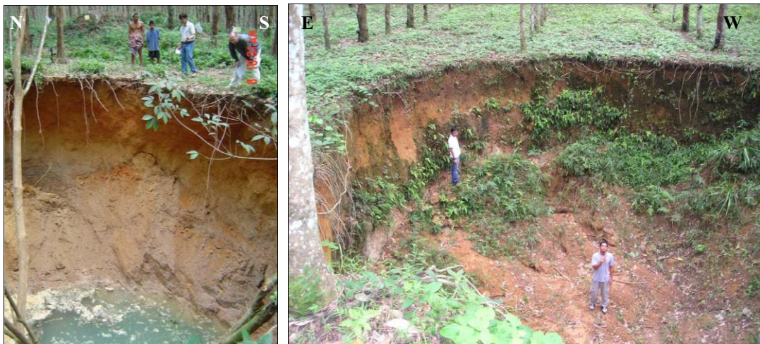
Figure 3.7 First sinkhole occurred in January 2005 (left) and later in June 2009 partly with clay filled in (right).
