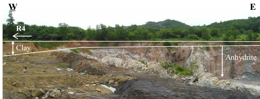
Figure 3.17 Subsurface structure from resistivity interpretation (top), which can be correlated to the geology survey around and inside the mine, a sandy clay layer overlay on the anhydrite. R4—resistivity survey point no. 4.
