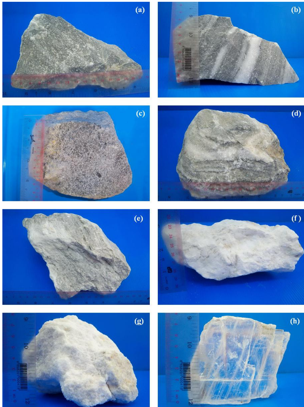
Figure 3.12 Photos of the rock samples from the gypsum mine with anhydrite of various weathering stages and structures, Sample (a) and (b); gypsum, Sample (c), (g) and (h), others might be anhydrite or gypsum or mixture of both.
