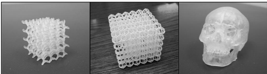
Figure 1.2: Examples of Rapid prototyping, showing geometrical freedom (Source: The National Metal and Materials Technology Center).
