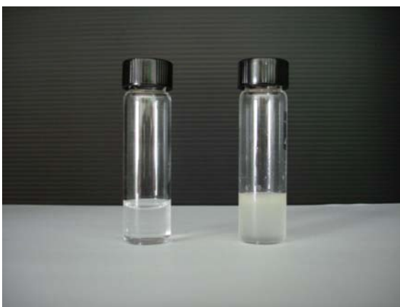
Figure 11. Determination of type of emulsion formed (a) filter paper wetting test and (b-1) dilution test of droplet in oil (b-2) dilution test of droplet in water.
