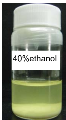
Figure 4.10 Physical appearance of the ethosome formulation prepared from 2% w/v SPC using 40% v/v ethanol in phosphate buffer pH 7.4 as dispersion medium
