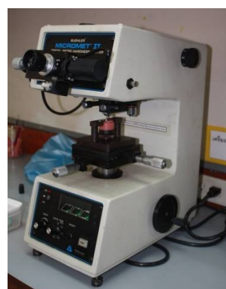
Fig.6 Knoop microhardness testing machine (Buehler Micromet II, Buehler, USA)
