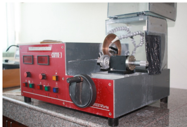
Fig.2 Slow cutting machine (JeanWirtz CUTO I, Wirtz-Buehler GmbH, Germany)
