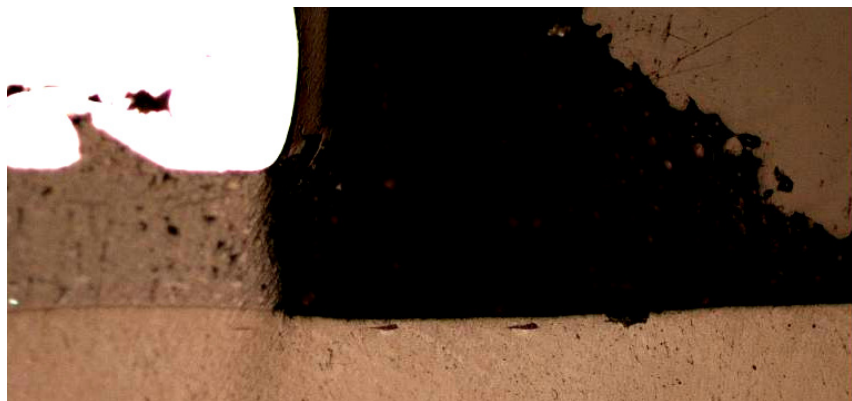
Fig. 7 Appearance under the Knoop microhardness tester at scale x100, bracket (upper left), acrylic resin (upper right) and enamel (lower)
