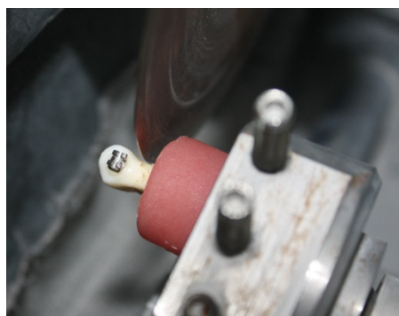
Fig. 3 The machine is cutting to separate the crown from the root
