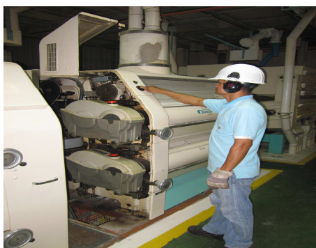
(D) Testing of feed rolling system after pneumatic equipment has been repaired
