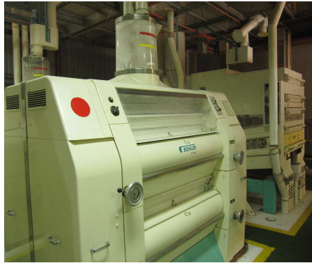
Figure 3.31 Identifying group of machine by color tag
