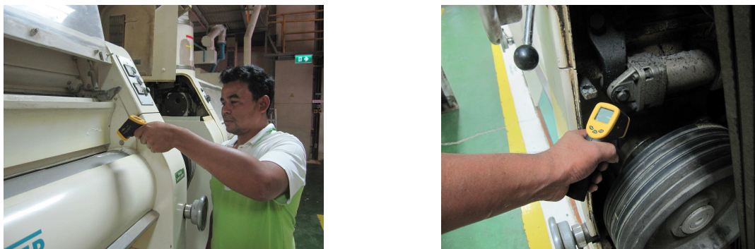
Figure 3.34 Checking machine temperature by infra - red temperature gun
