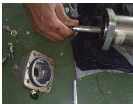
(B) Repairing of grinding roller cylinder
