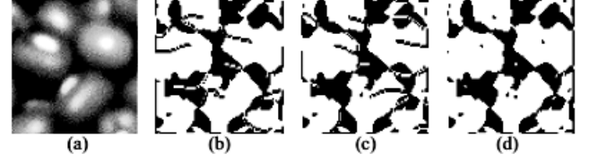
Figure 3. (a) The original image. (b) The binary image from the binarization of \Delta\omega(x, y, \nu = x) . (c) The binary image from the binarization of \Delta\omega(x, y, \nu = -x) . (d) The corrected binary image.
