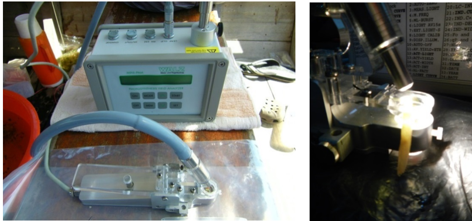
Fig. 22 Photosynthetic measurement by RLC method was performed using PAM fluorometry in dark-adapted leaves of the seagrass H. ovalis .
