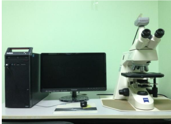
Figure 9. A microscope (Axiostar, Carl Zeiss, Göttingen, Germany) coupled to a high resolution digital camera (AxiocammRC, Carl Zeiss)
