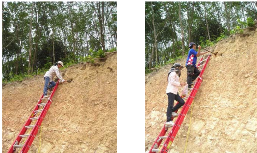
Figure 2.3 Sampling of unconsolidated sediments using standard tools (left) with the samples afterwards put in a plastic bag (right).
