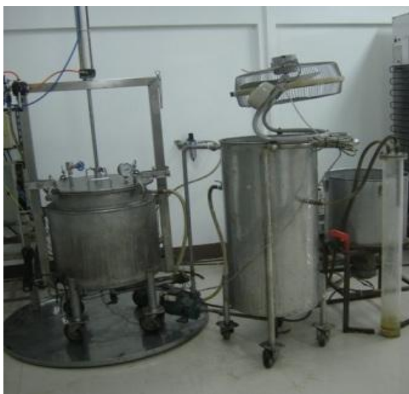
Figure 32 Photograph of vacuum drying system
