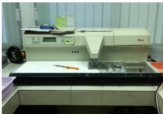
Figure 12. Paraffin Embedding Station; EG 1160; Leica; Germany
