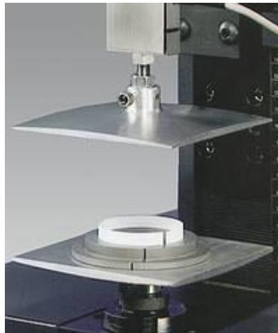
Figure 2.7 Ring crush test for measuring the resistance of paper to the compression force.
