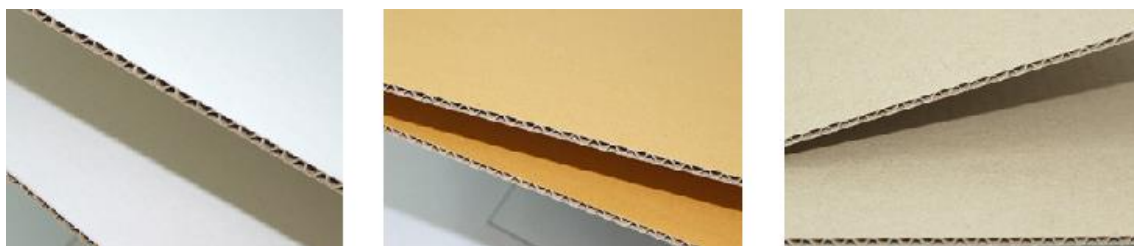
Figure 2.5 Major grades of Kraft linerboards; KS (left), KA (middle), KI (right) [11].
