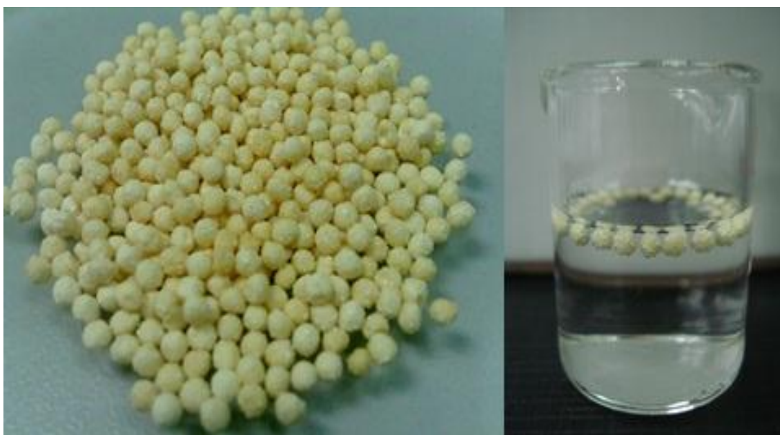
Figure 3.17 The THC-SME floating calcium alginate beads are almost spherical (left) and still float in SGF (pH1.2) after 8 h (right).
