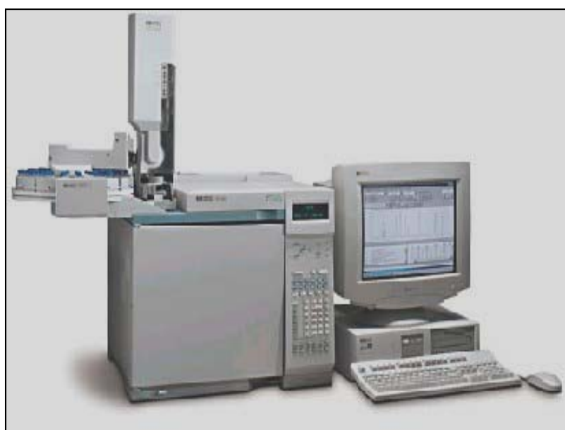
d. Gas Chromatography with ECD detector control by computer (Agilent 6890 Series Gas Chromatography).
