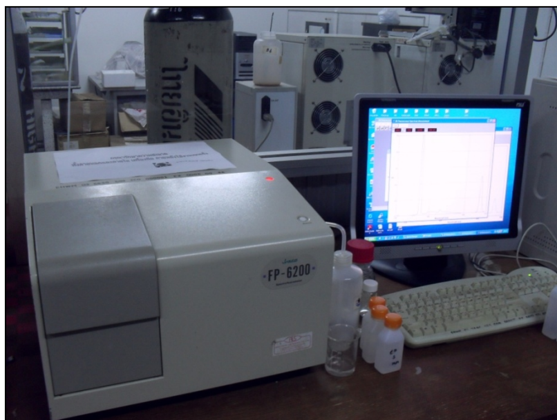
b. Spectrofluorometer (FP-6200 spectrofluorometer from JASCO)
