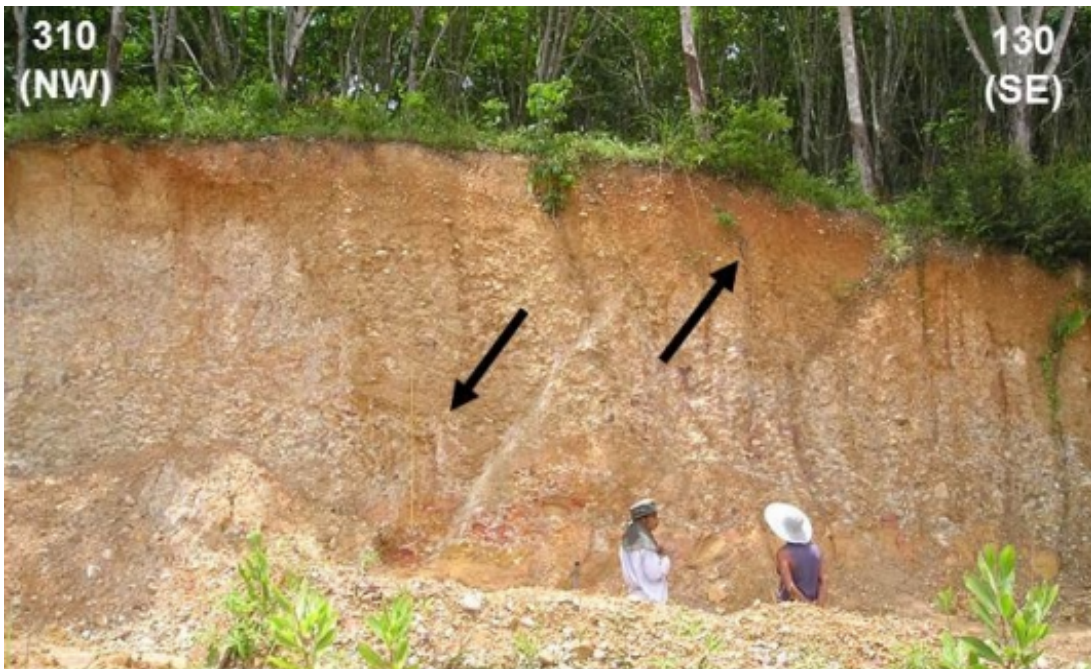
Figure 3.9 Site V3: Fault with white clay apparent on the plane with an orientation of 282/55 (dip direction/dip angle) and a vertical movement of about 50 cm.
