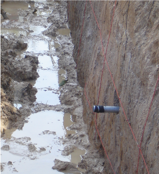
Figure 3 TL sampling with a steel pipe in a trench (photo here taken at day light).
