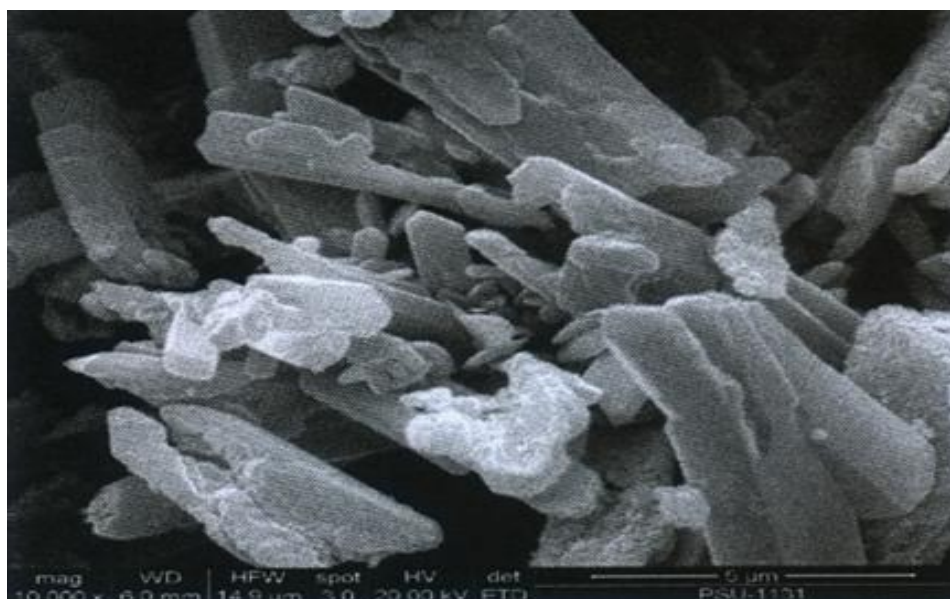
Figure 3.2.2.3 SEM image of BTO at 10,000X magnification
