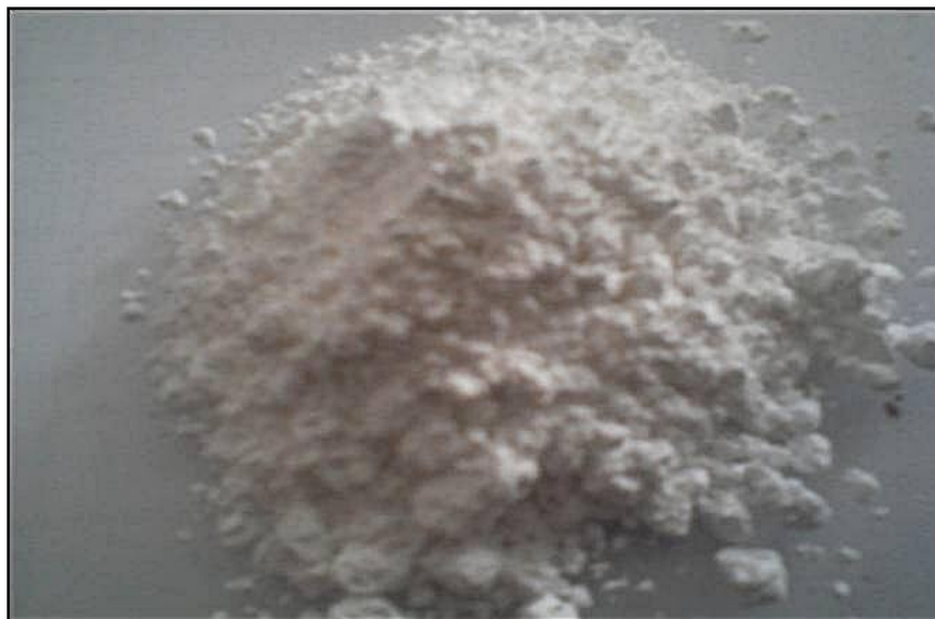
Figure 3.1.5 \text{TiO}_2\text{-BaC}_2\text{O}_4 obtained from synthesis
