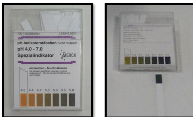
Fig.3: The pH-indicator strip for determination of salivary pH value
