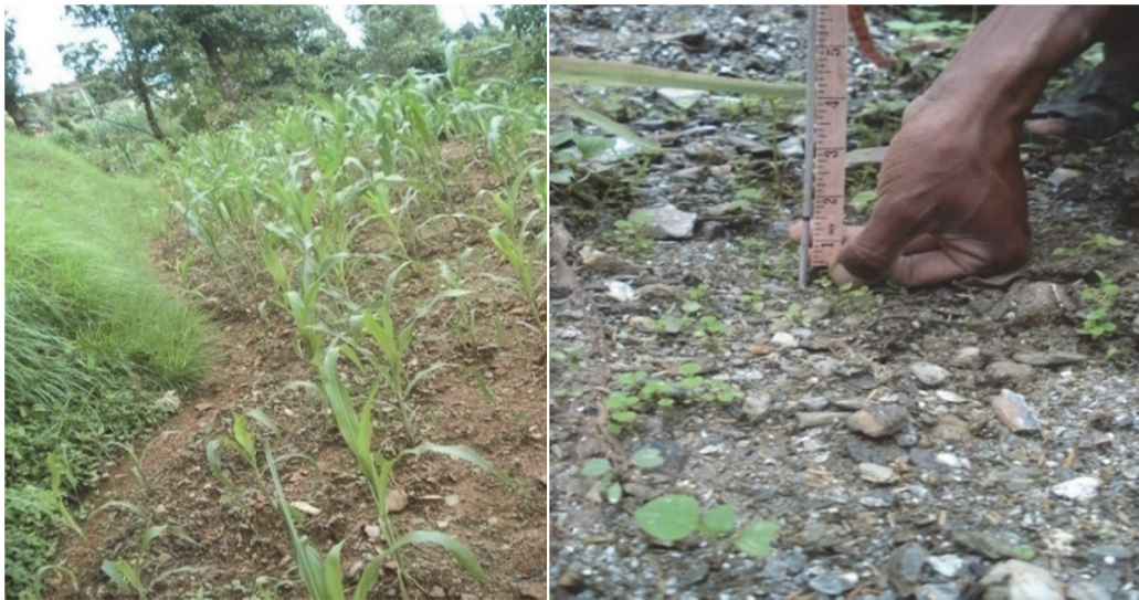
Figure 44 Maize Plot Erosion Feature and Rill Dimension Measurements of Barren Land after Rainfall
