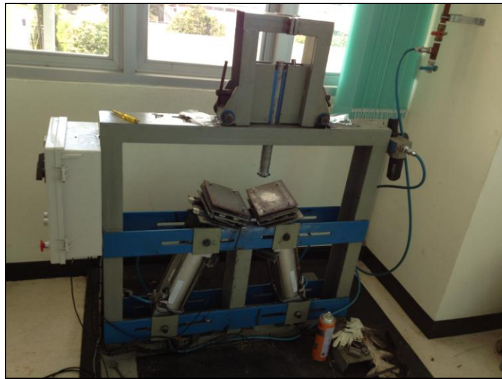
Figure 3-13 The modified gauge machine for device fatigue test
