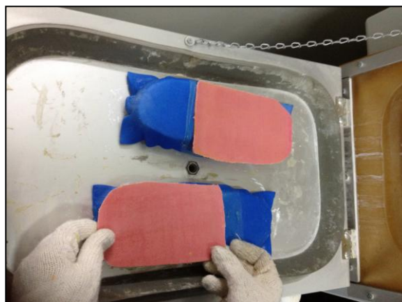
Figure 3-26 The soft composite plate on the positive mold
