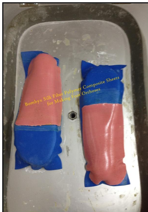
Figure 3-28 The setting in the form of foot orthoses of composites
