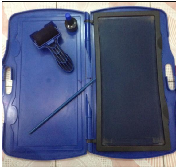
Figure 2-7 Rubber layer and plastic base impregnated with regular stamp ink for capturing footprints
