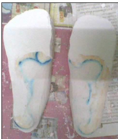
Figure 3-20 Finishing Positive Foot Mold
