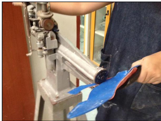
Figure 3-31 Cut the trimlines
