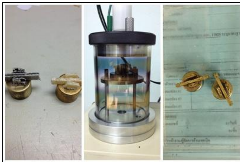
Figure 3-15 Composite preparation and gold coated for SEM analysis
