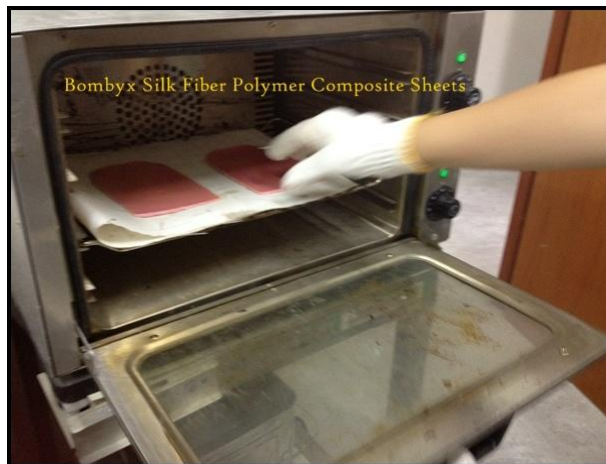
Figure 3-25 The composite in the heat oven
