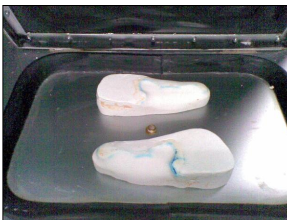
Figure 3-22 Positive mold on the vacuum press
