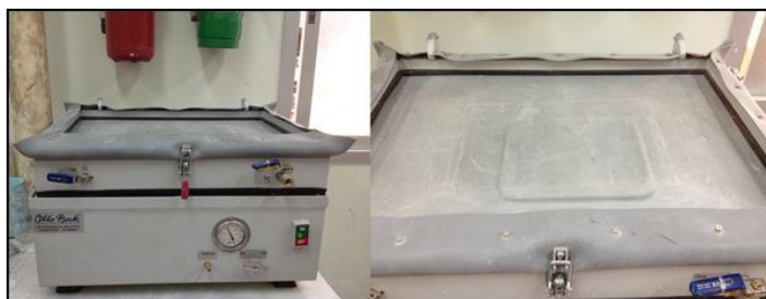
Figure 3-3 Vacuum machine (left) and the chemical action of composite making on vacuum machine (right)
