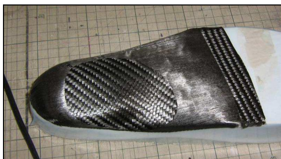
Figure 1-2 Laying up Process [36]
