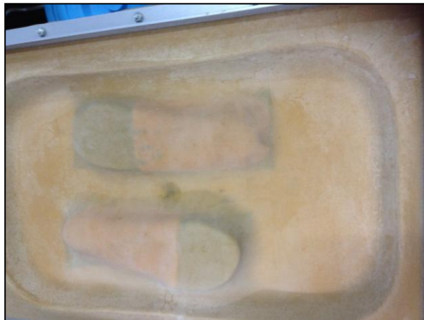
Figure 3-27 The vacuum press machine suck the air out to attach the positive mold
