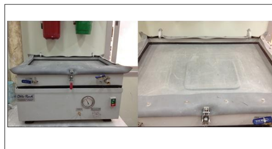
The picture of vacuum machine (left) and the chemical action of composite making on vacuum machine (right)
