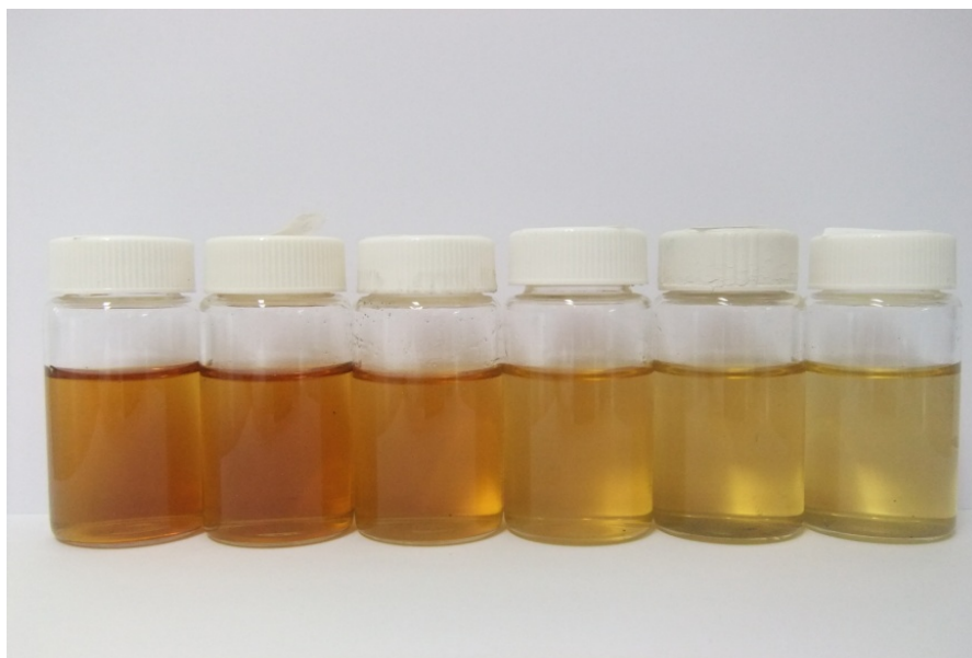
Figure 13. Comparison on color of final effluent before by using 0, 1, 5, 10,15 and 20 % (w/v) palm ash, respectively
