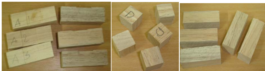
Compression strength parallel to grain Shearing strength Compressive strength perpendicular to grain
