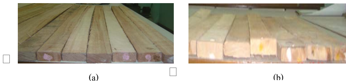
□ Figure 4-5. Physical property resulted: (a) After drying with impinging hot-air at 70°C, □ (b) After drying with impinging hot-air at 80°C
