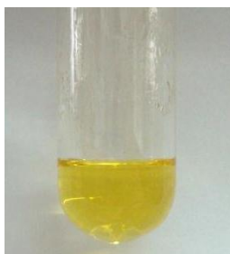
Latex digestion with nitric acid and hydrogen peroxide
