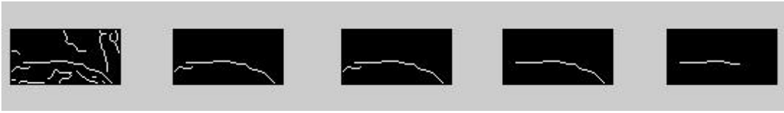
Figure 28. Canny edge detector outputs for a right eyebrow image, with values of 0.1, 0.3, 0.5, 0.7, and 0.9.
