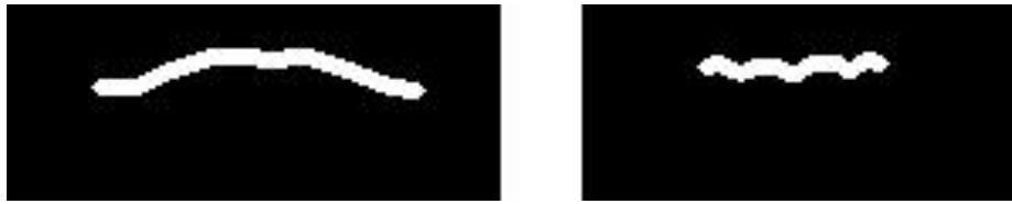
Figure 33. Lips edge detection on neutral and peak frames for a happy expression from CK+. Edges in the first frame were found correctly, but the presence of teeth in the second frame produced edges that resulted in an incorrect detection of lips.
