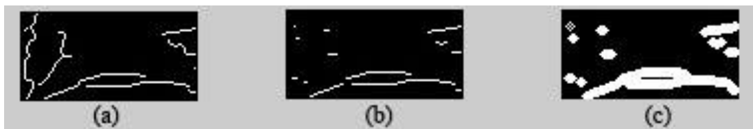
Figure 30. Example of left eyebrow edge detection with: a) Canny edge detector, b) after removing vertical edges, and c) after re-connecting the edges.
