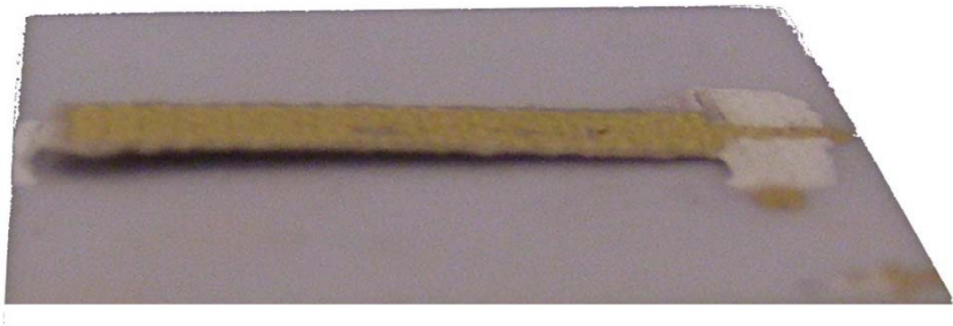
Figure 6.13 The BZT (group A) cantilever of the element of dimension of 10 \times 2 \text{ mm}^2 thickness \sim 60 \text{ }\mu\text{m} .
