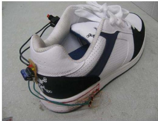
**Figure 5.7** Complete shoe with transducer inserted in the heel and capacitor circuit attached. (Fourie,2009).
