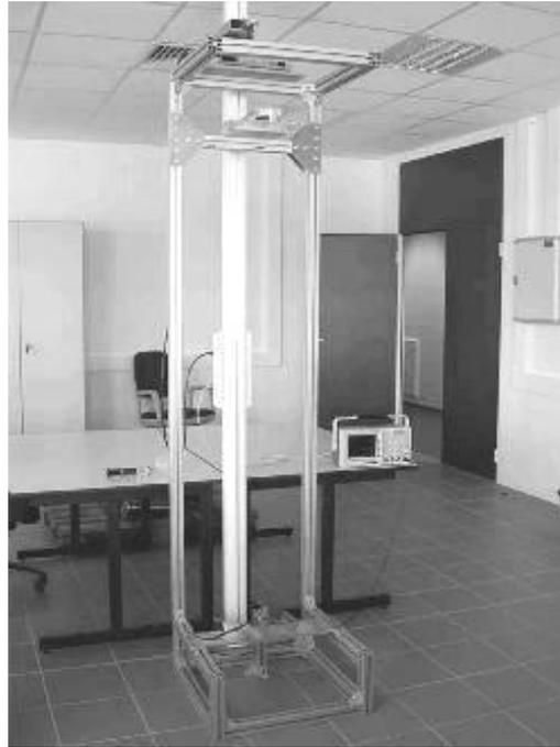
**Figure 5.9** Testing apparatus of capturing energy from raindrop
