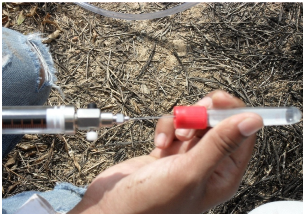
Figure 4.5 The gas samples were collected by gas tight syringe in vacuum tube.
