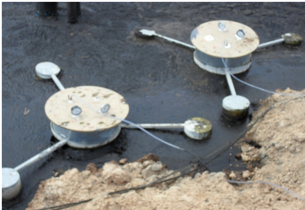
Figure 4.4 Close flux chambers put on surface area with/without scum layer.
